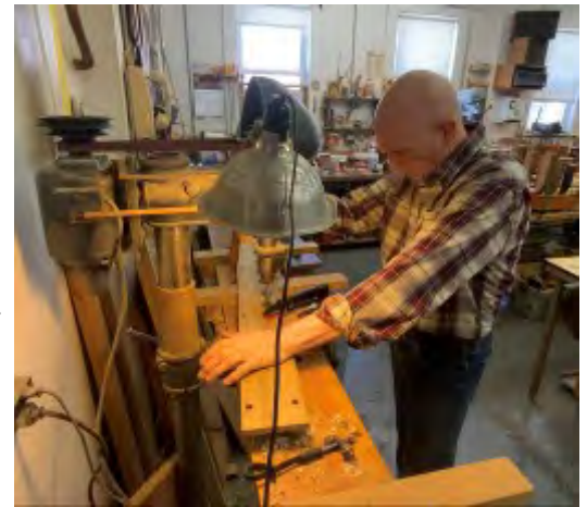
Jon Van Houten fabricating a new rack board for the Casavant organ at the workshop of Czelusniak et Dugal in Northampton.
